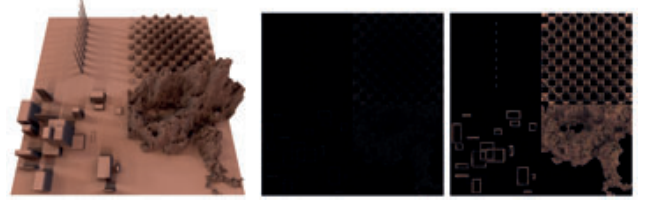
Figure 7: Error introduced by lowering the normal angle resolution from a reference 256 to 16 (middle) and 8 (right) on a height field shown to the left, multiplied by 50. The average and maximum errors for resolution 8 are 0.16% and 1.66%, and for resolution 16 0.03% and 0.42% respectively.
