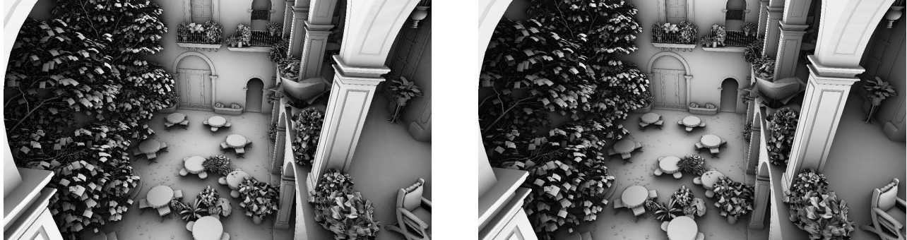
Figure 1: Left: screen-space far-field ( \geq 15 px) occlusion component solved by our method in 4.6 ms on a 1280(+256) \times 720(+144) depth buffer. Right: ray traced screen-space reference result.
